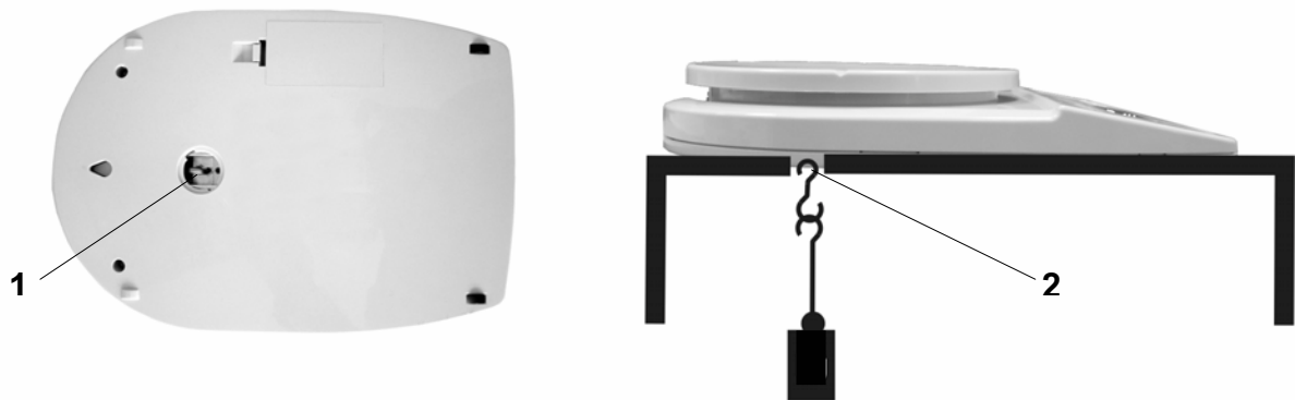
Fig. 1: Setting up the balance for underfloor weighings
